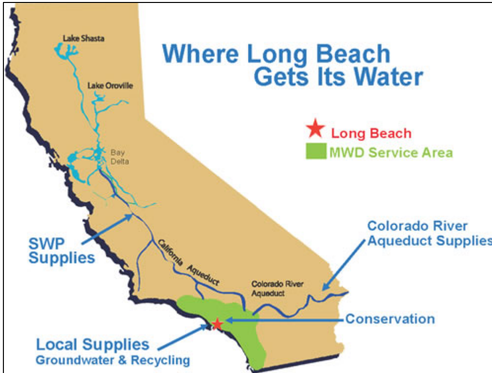
Figure 2-2. LBWD Water Supply Sources
