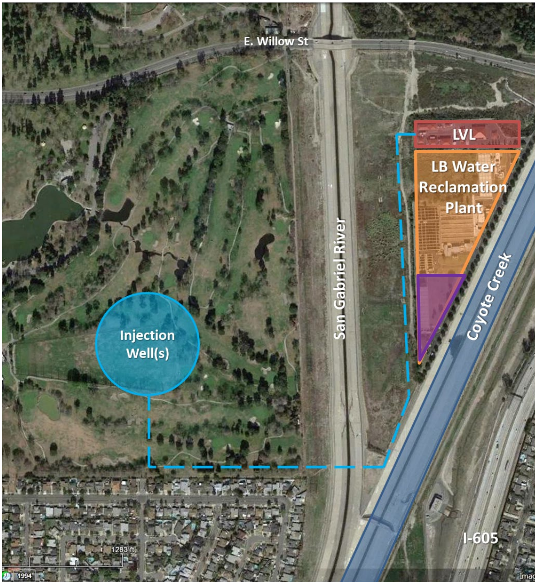
Figure 6-5. Pipeline Alignment for LVL Injection
