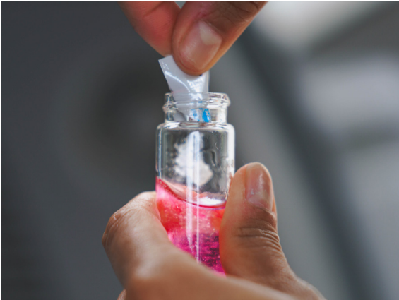
Pictured: A water sample with a powdered reagent (called DPD) added to see the concentration of chlorine in the sample
