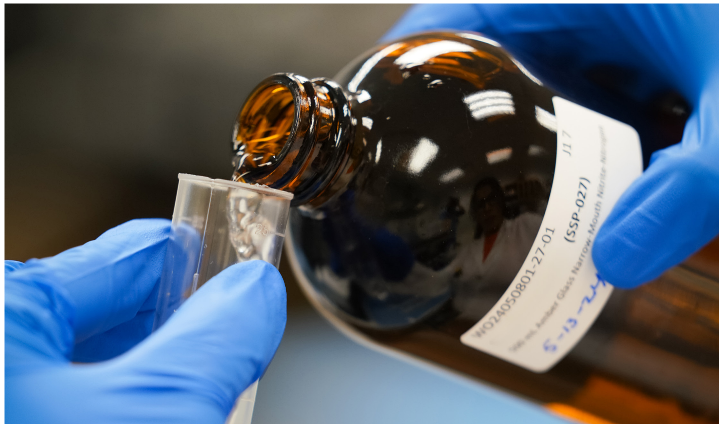
Pictured: An aliquot of water is poured from a sample bottle into a sample cell for ammonia analysis
