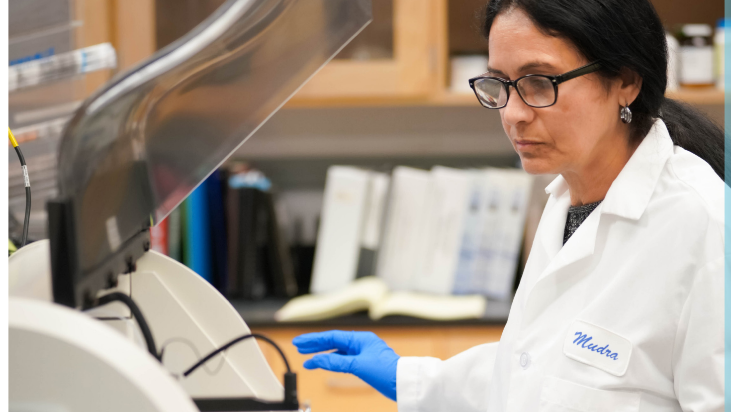
Pictured: Mudra, a LBUD laboratory analyst, loads samples for nitrite analysis on a discrete analyzer
