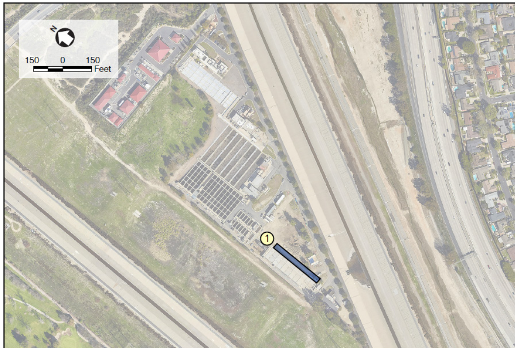
① New Chlorine Contact Tank (287.5'x20')
